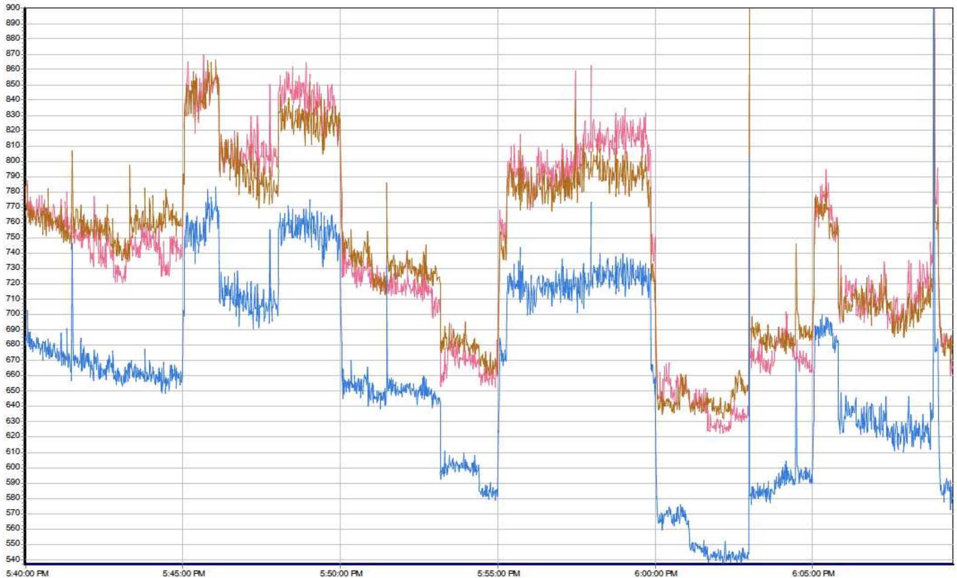
Graph 5B Above shows the Current in Amps per phase during the TIS testing on July 21, 2011 between 5:40 pm and 6:09 pm. With 4 USES ® model CMES 240V and 5 USES ® model CMES 460V power conditioners operating, the current is reduced an average of 90.24 Amps per phase.
