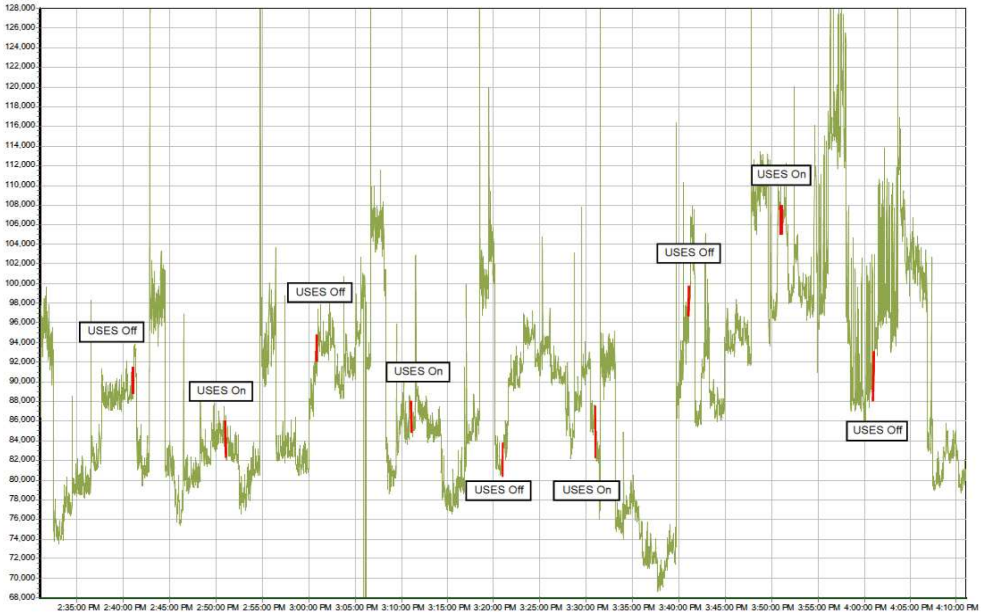
Graph 1A Above shows the Real Power Demand in watts during the TIS testing on July 21, 2011 between 2:31 pm and 4:11 pm. With 4 USES ® model CMES 240V power conditioners operating, the real power demand is reduced an average of 4,763.13 watts .
