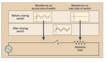
Fig. 1 also shows the switch closing just as the voltage waveform crosses zero. This is the preferred time of closing. If the switch closes at
