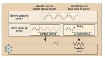
physics state that neither the current flow through an inductor nor the voltage across a capacitor can change instantaneously. In reality, some inductance and some capacitance are present in all circuits, although the values may be very small.
