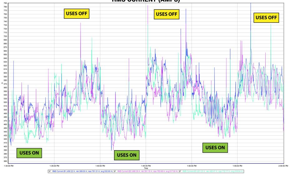
GRAPH 5A above shows RMS CURRENT (AMPS) during Timed Interval Sampling (TIS) Testing on April 5, 2012 between 1:30:00 PM and 2:00:00 PM of a fully operational USES® System installed at the Roll-Kraft manufacturing plant. The USES® System consists of (1) USES® CMES-Y-480V UNIT and (4) USES® CMES-D-480V UNITS. The graphical test result above shows a REDUCTION in RMS CURRENT (AMPS) of 81.56 Amps for the six (6) interval periods.
