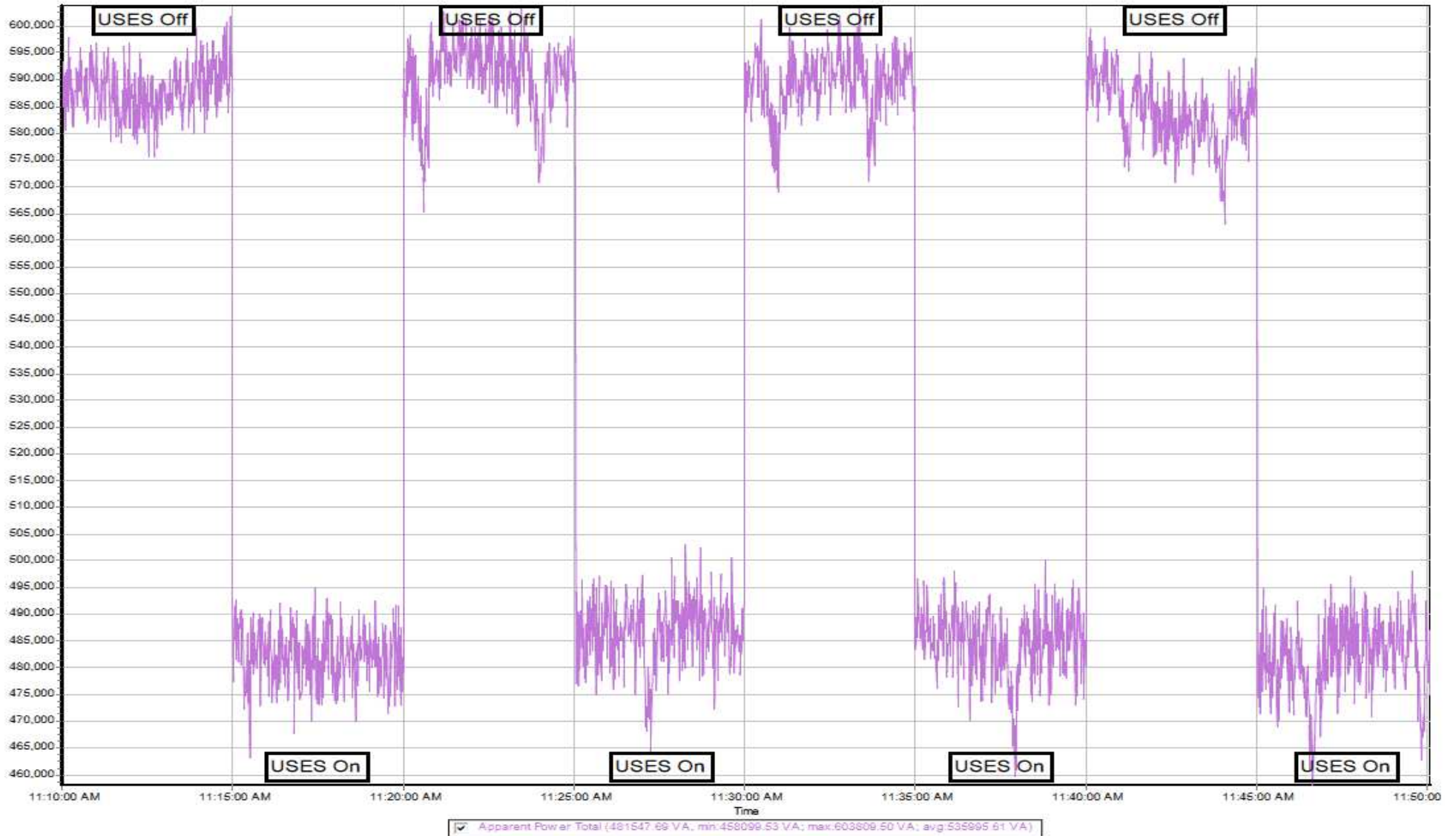
Graph 2 Above shows the Apparent Power in VA during the TIS testing on August 15, 2012 between 11:10 am and 11:50 am with eight (8) USES ® model CMES-3D-480V and one (1) USES ® model CMES-3Y-480V power conditioners operating. The Apparent Power is reduced an average of 104.23 KVA .
