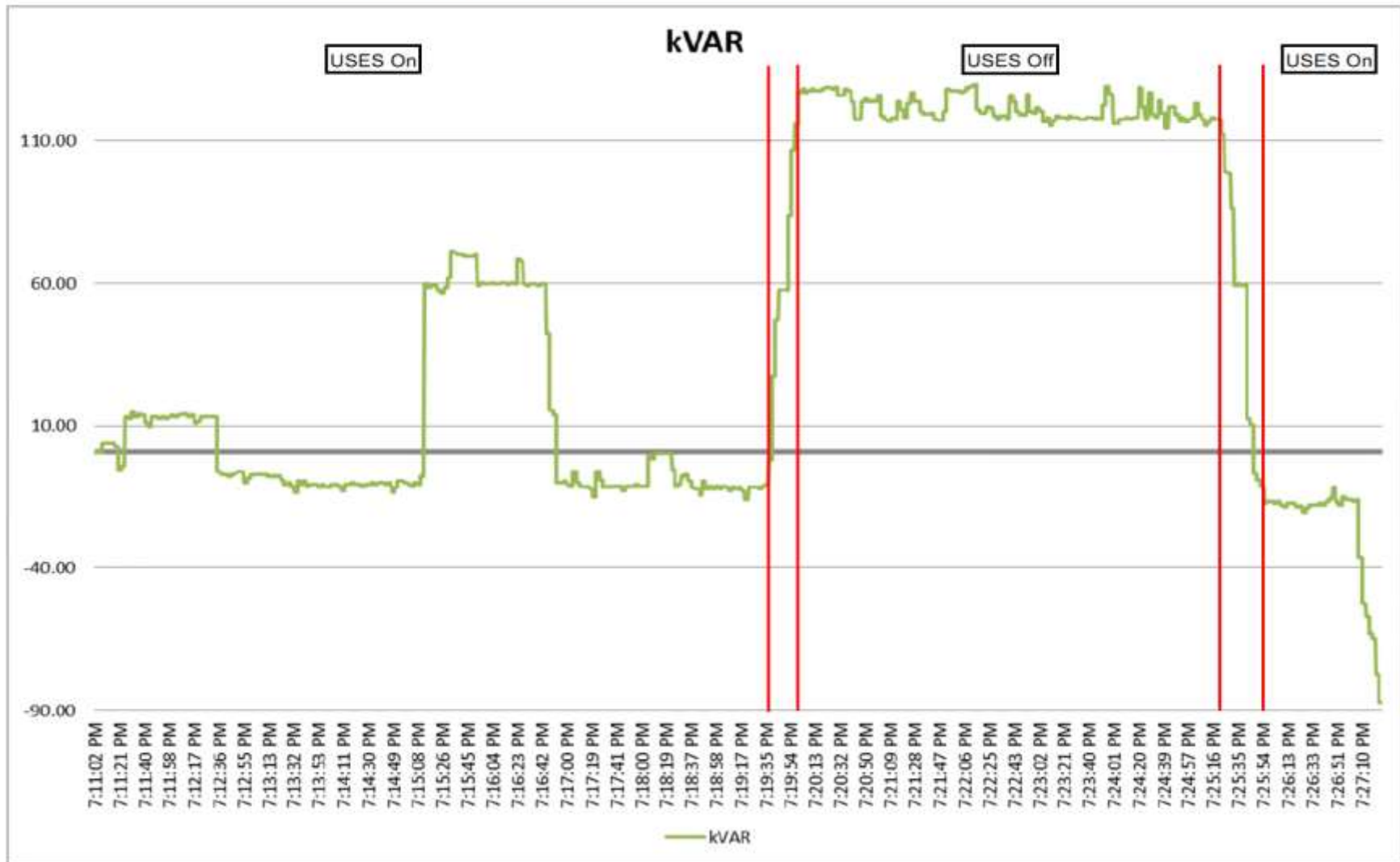
Graph 3 above shows the Press Reactive Power in kVAR during the TIS testing on February 23rd 2016 between 7:11pm and 7:27pm. With (3) USES® model XL-3D-480V and (1) USES® model XL-3Y-480V power conditioners operating. The reactive power is reduced an average of 122.75 kVAR .
